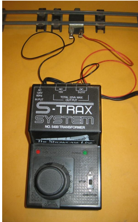
Figure 2: DC Power Source connected directly to the track
