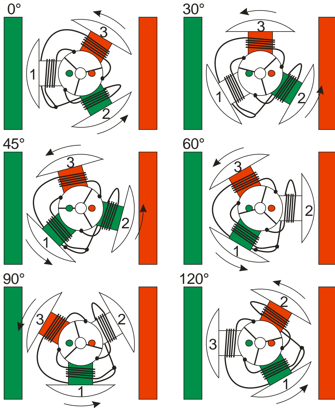
Figure 77: Common Tie-Off Rotor Reverse Direction
