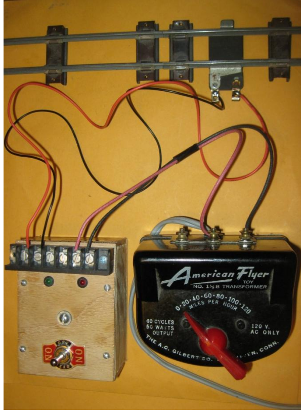
Figure 4: AC Transformer with Rectifier to provide DC to the track
