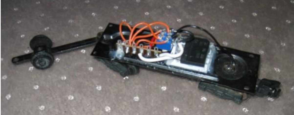
Figure 8: Rectifier and Reverse Switch in a tender
