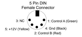
Note: If either the Straight or the Curved Inputs are grounded, then the appropriate coil on the switch is energized. If both inputs are grounded, the switch coils are not energized.
