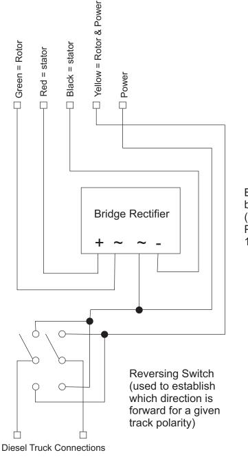
Bridge Rectifier should be rated at least 4 amps (5 or 6 is better) with a PIV rating greater than 100 Volts
