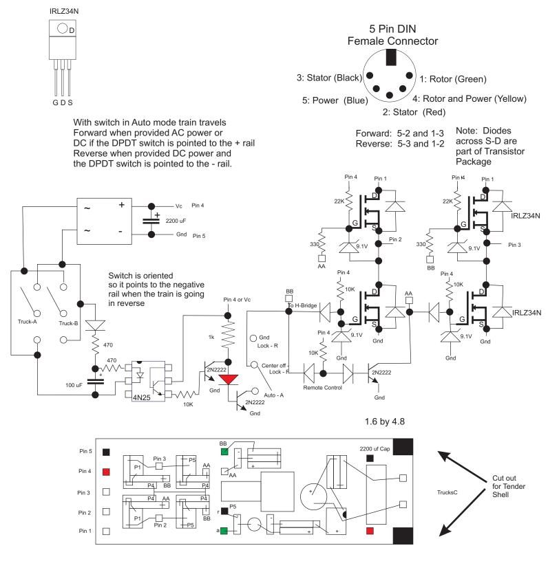
Power FET (n channel) Based AC-DC Reversing Unit Rev 1 Norbert Doerry Dec 2011
