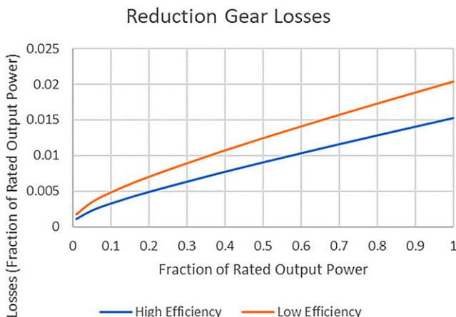
Fig. 5 Reduction gear losses
