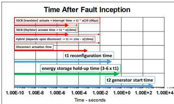
Fig. 7, MVDC fault protection duration times
