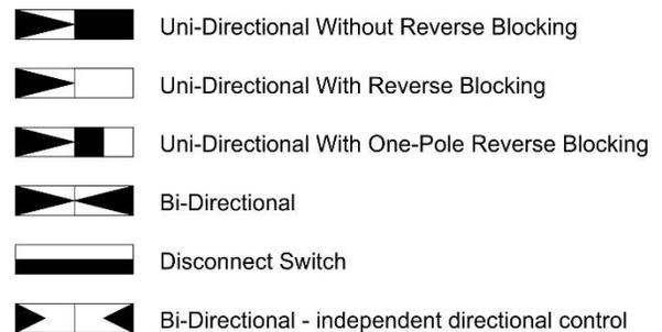
Fig. 4, Recommended symbols for different types of protection devices
