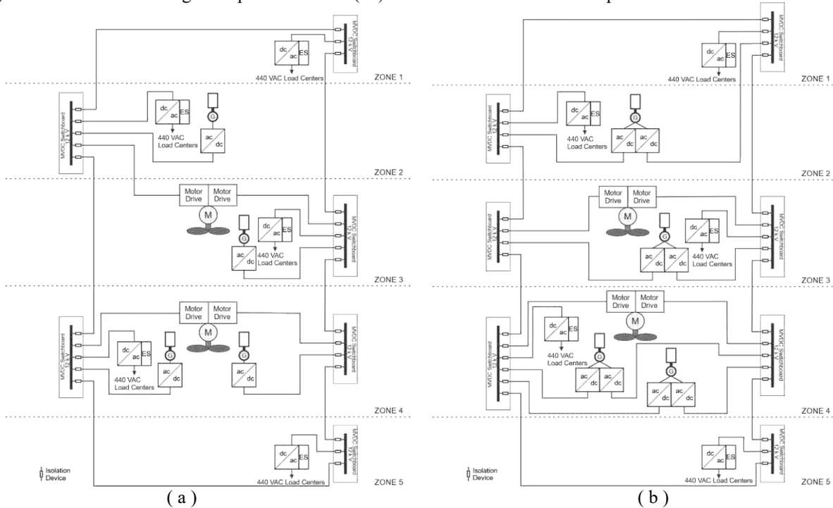
Fig. 2, ( a ) Zonal Distribution Single Output Generators ( b ) Zonal Distribution Dual Output Generators
