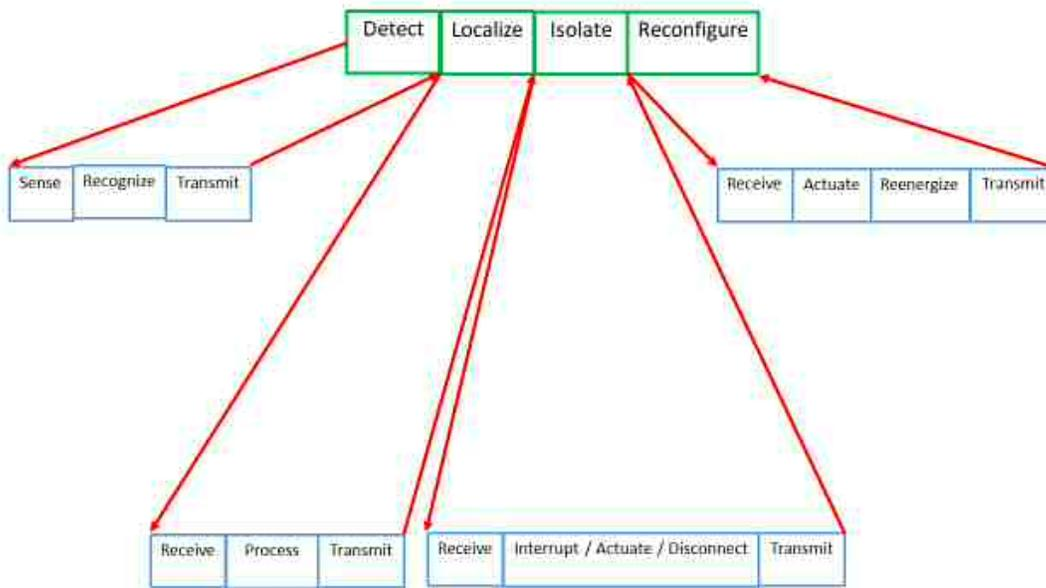
Fig. 6, Activities within MVDC fault protection timeline
