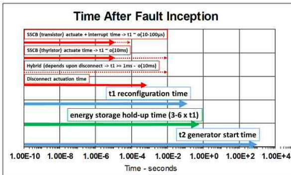
Fig. 7, MVDC fault protection duration times
