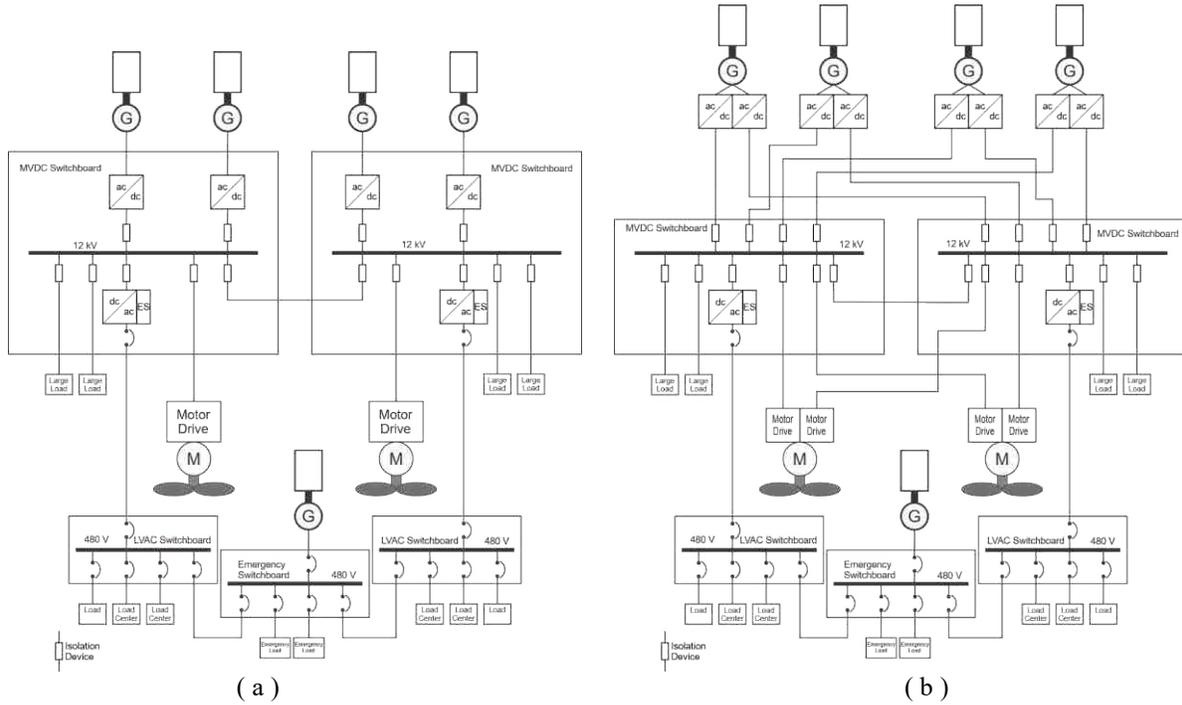
Fig. 1, ( a ) Radial Distribution Single Output Generators ( b ) Radial Distribution Dual Output Generators
