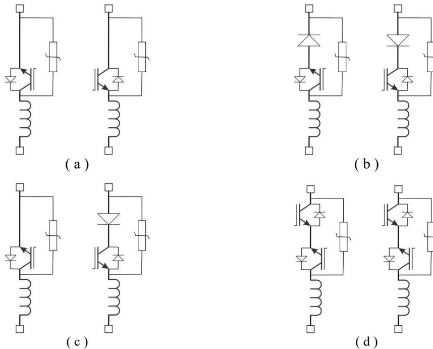
Fig. 3, SSCB directional functionality (a) unidirectional without reverse blocking (b) unidirectional with reverse blocking (c) unidirectional with one pole reverse blocking (d) bidirectional (with independent directional control).
