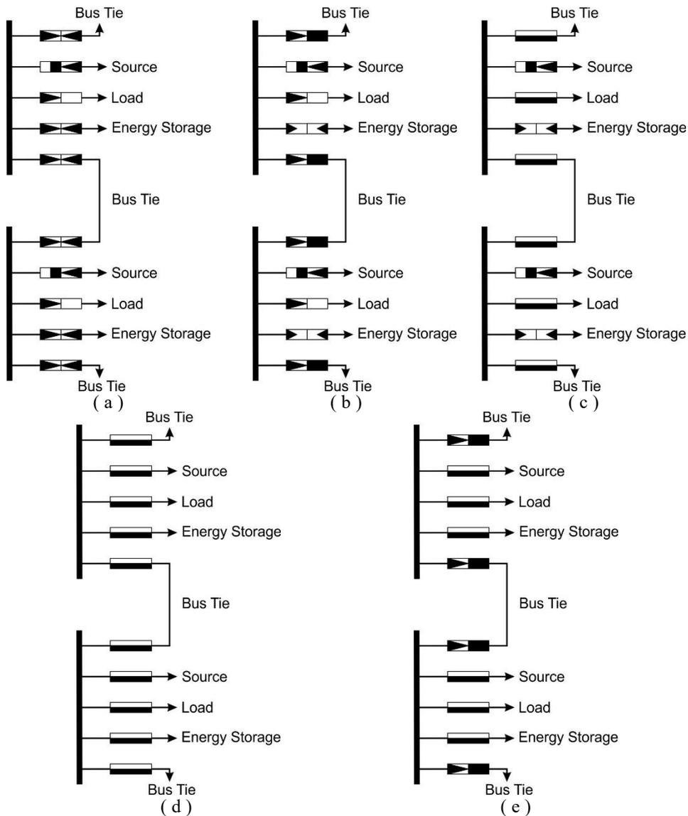
Fig. 5, Isolation device strategies for MVDC fault protection
