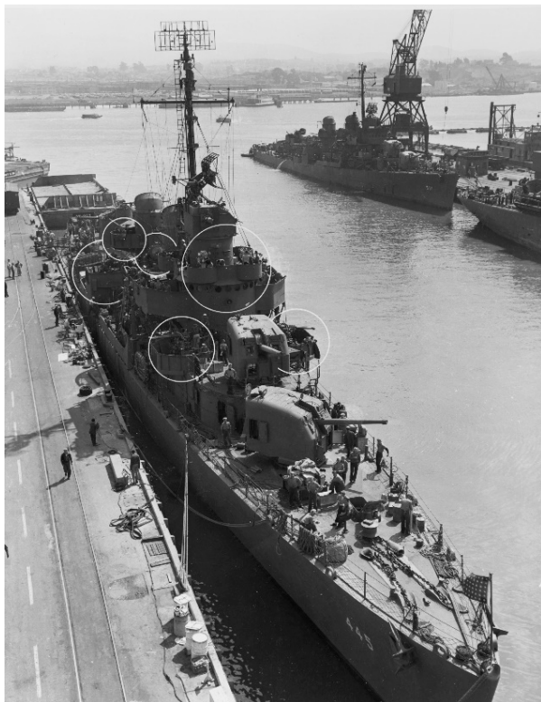
Fig 3. USS Fletcher (DD 445) at Mare Island Navy Yard on 13 August 1943. Circles mark alternations including the addition of Bofors twin mounts. (www.history.navy.mil – 19-N-50812)
