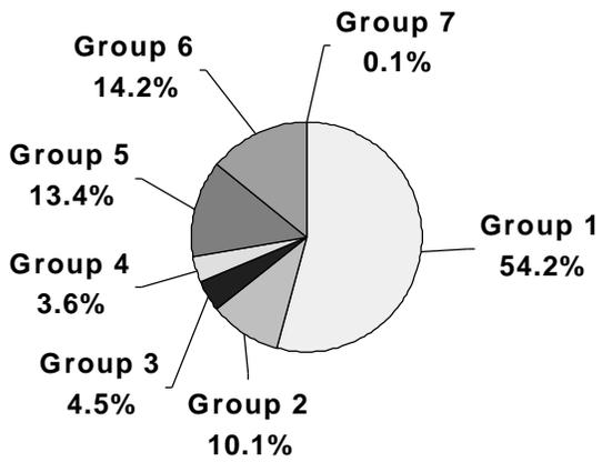
**FIGURE I-2: Typical JCC(X) SWBS Weight Fractions**
