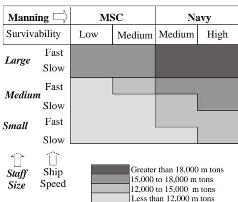
**FIGURE 2: Example of Design Space Study results – Light Ship Displacement**
