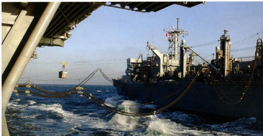
The fast combat support ship USNS Arctic (T-AOE 8), right, transfers fuel while sending supplies and other stores to the Nimitz-class carrier USS Harry S. Truman (CVN 75) via cable during underway replenishment in the Persian Gulf in 2004. United States Navy photo by Photographer's Mate Airman Kristopher Wilson.
