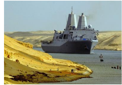
Figure 7: USS San Antonio (LPD 17) – note advanced enclosed masts – transits through the Suez Canal. U.S. Navy photo/Released, 080923-N-1082Z-038)
