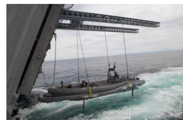
Figure 9: A rigid-hull inflatable boat is hoisted onto the littoral combat ship USS Coronado (LCS 4) (U.S. Navy photo/ Released, 170219-N-WV703-239)
