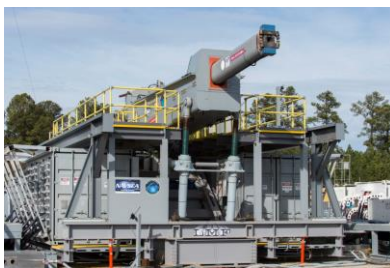
Figure 2: Electromagnetic Railgun at terminal range located at Naval Surface Warfare Center Dahlgren Division. (U.S. Navy photo/Released, 170112-N-PO203-142)
