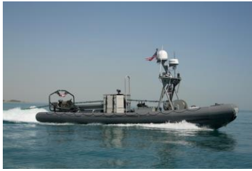
Figure 10: Sailors and civilian personnel remotely pilot an unmanned surface vehicle (USV) from ashore several miles away as the USV deploys an AQS-24A sonar (U.S. Navy photo/Released, 160417-N-QG671-003)
