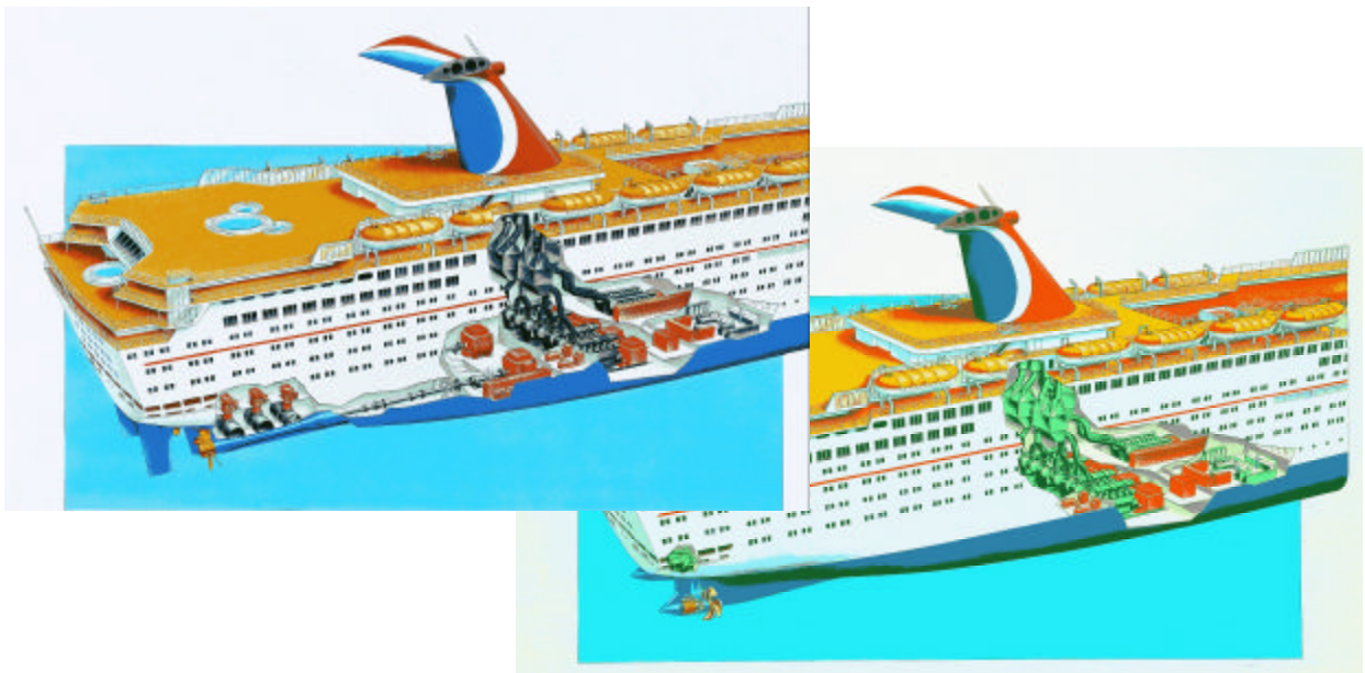
Fig. 1.5: Cruise vessel "M/S Elation" (lower right) equipped with Azipod propulsion frees up space compared to sisterships (upper left) that can be utilized for other purposes, e.g. grey water treatment.
