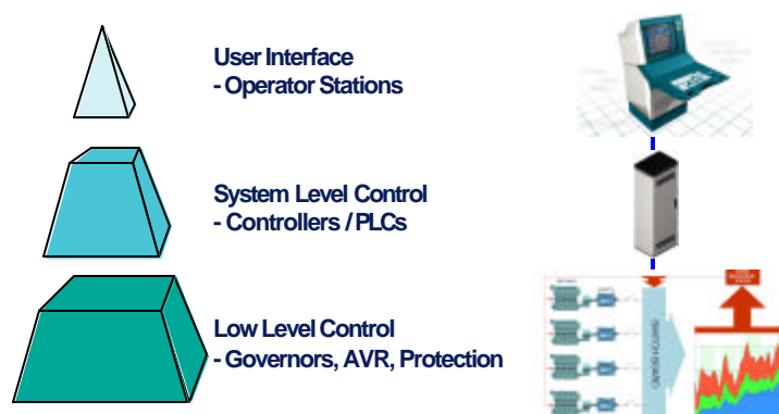
Fig. 4.2: Control Hierarchy for a Power Plant
