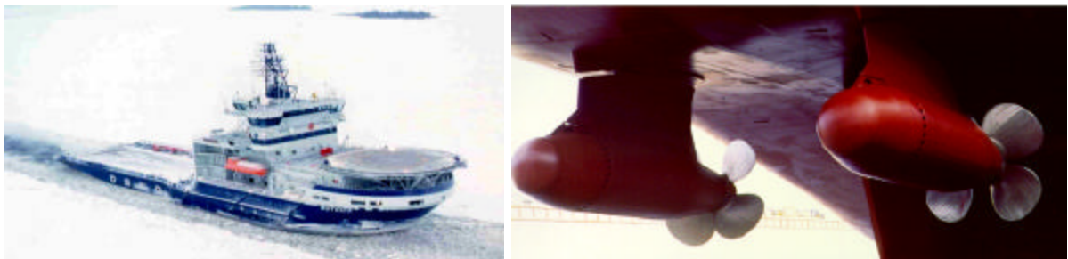
Fig. 2.5: "M/S Botnica", Icebreaker which serves as a supply vessel in summer season, equipped with Azipod propulsion.
